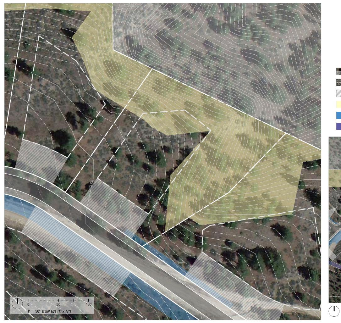
Parcel Boundary Building Envelope Driveway Location(s) Slope Constraints (+25%) Drainage Easements IVGID Easement
